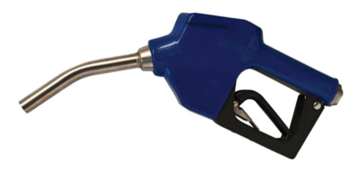
Automatic Shut Off Stainless Steel Body + Spout 3/4" BSP Female Inlet Viton Seals
