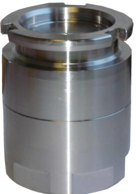
The Atkinson dry break coupling for ADBLUE is designed to open and close automatically when the delivery hose is connected and disconnected. The valve insures minimal liquid loss on disconnection even if connected or disconnected whilst filling is in progress
